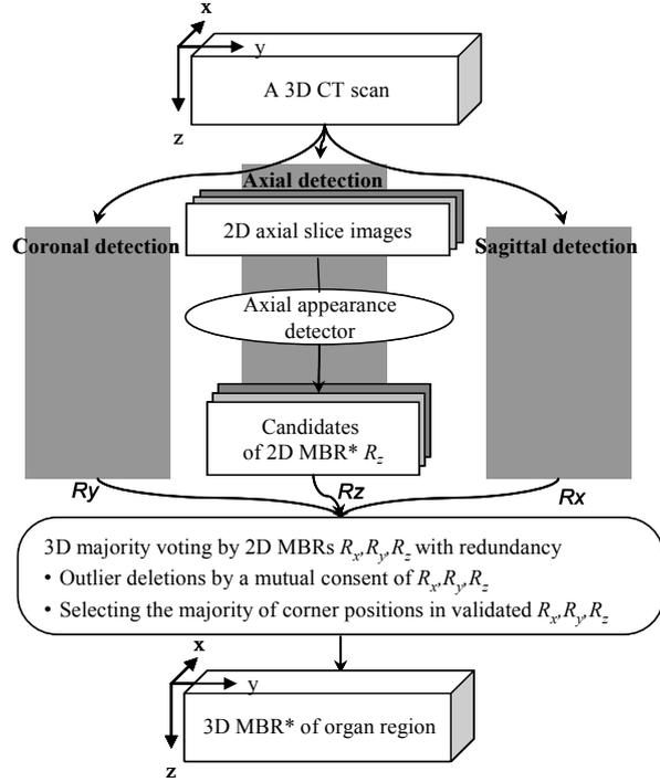
**Fig.1.** Process flow for localizing a solid organ in a 3D CT scan. (\*MBR: minimum bounding rectangle)
